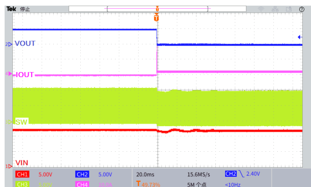
Figure22. Output Short Circuit Waveform ( V_{IN}=12V , V_{OUT}=5.0V )
