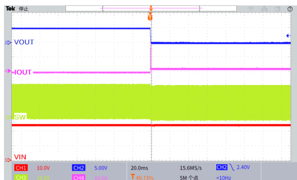
Figure23. Output Short Circuit Waveform ( V_{IN}=24V , V_{OUT}=5.0V )
