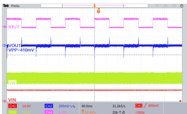
Figure30. Load Transient Response ( V_{IN}=12V , V_{OUT}=5.0V , I_{OUT}=0.1 to 1A )
