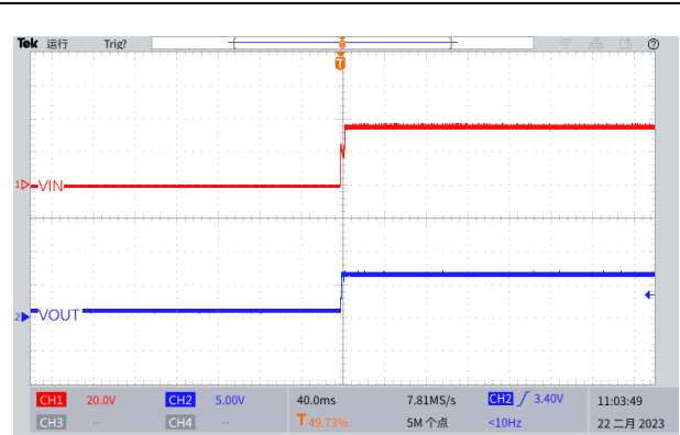
Figure26. Start-Up Characteristic ( V_{IN}=36V , V_{OUT}=6.6V , I_{OUT}=0.3A )
