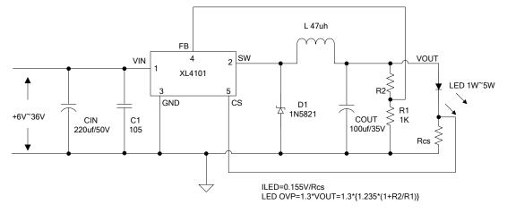
Figure 5. XL4101 Typical Application Circuit (LED Constant Current Driver)
