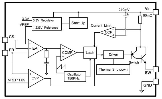
Figure 3. Function Block Diagram of XL4101
