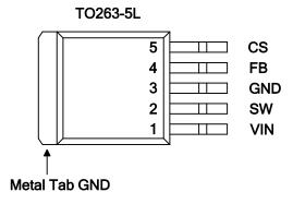
Figure 2. Pin Configuration of XL4101 (Top View)
