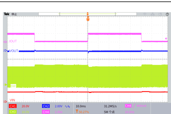
Figure 25. Load Transient Response ( V_{IN}=24V , V_{OUT}=12V , I_{OUT}=0.1 to 1.0A )
