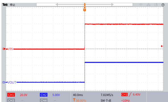
Figure 18. Start-Up Characteristic ( V_{IN}=60V , V_{OUT}=12V , I_{OUT}=0.1A )
