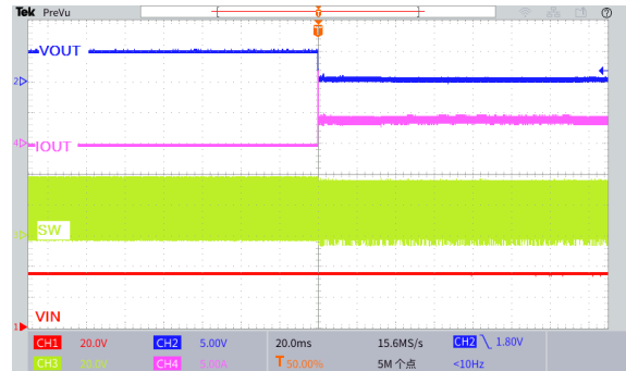
Figure 25. Output Short Circuit Waveform ( V_{IN}=36V , V_{OUT}=5.0V )
